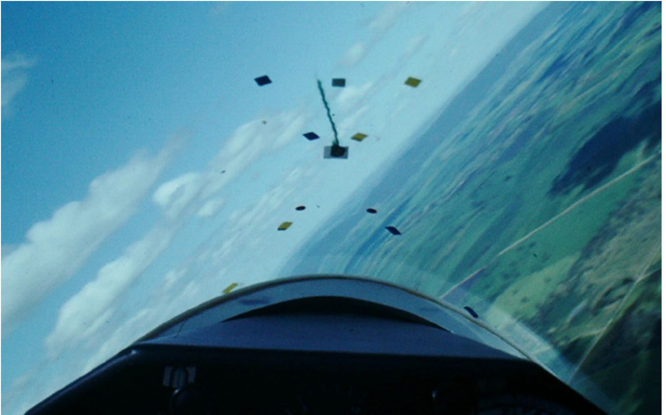
Pitch wrong (nose too high) , roll correct (45°), yaw wrong (slipping)
