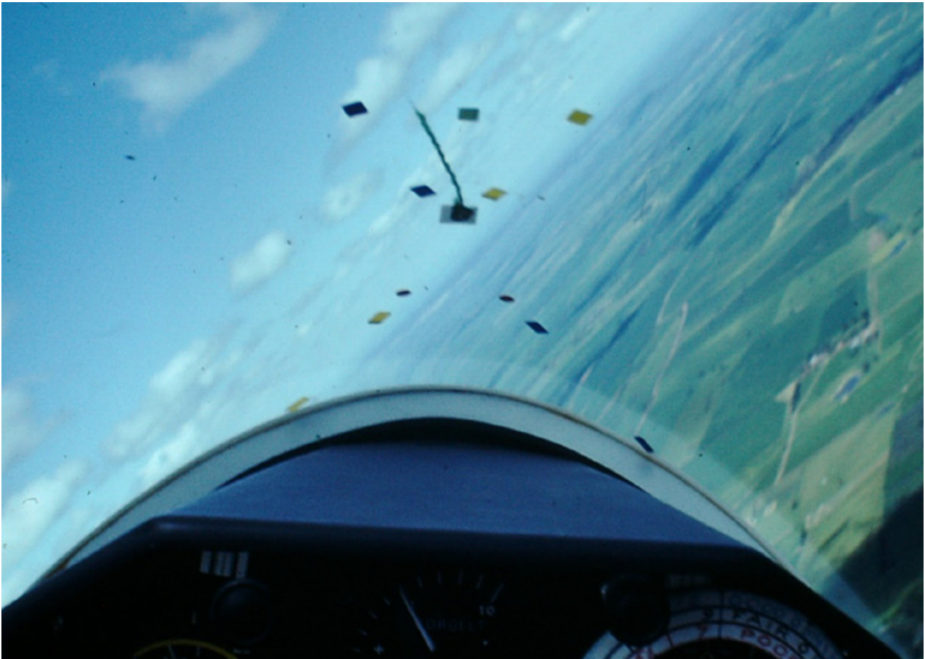
Pitch correct for 50 knots, roll correct (45°), yaw wrong (slipping)
