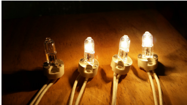
Battery Test Rig - 14 Watt 2Pin Halogen lamps provide a Battery load of 1.2Amps
