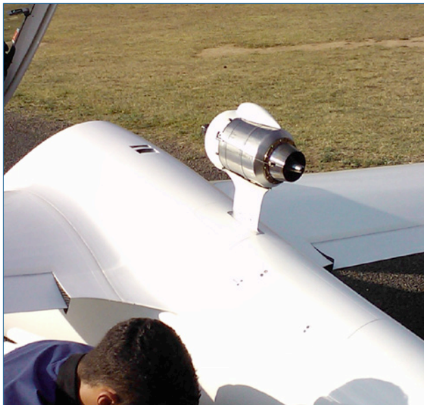
A neat installation - the engine bays doors closed with motor extended. Fairings over the motor support and controls, and the fibreglass nose cone all minimise aerodynamic drag. "Any increased drag was not noticeable. It seemed to be less than the drag from the undercarriage."
