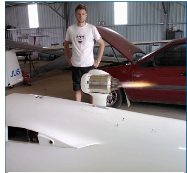
During start up there is a short impressive fiery display out the back of the jet which disappears as ignition burn is fully established. The motor is offset from the centreline by 4° so the exhaust misses the fin. Even so, you can comfortably stand in the jetstream alongside the fin, and when flying the airstream provides further cooling.
