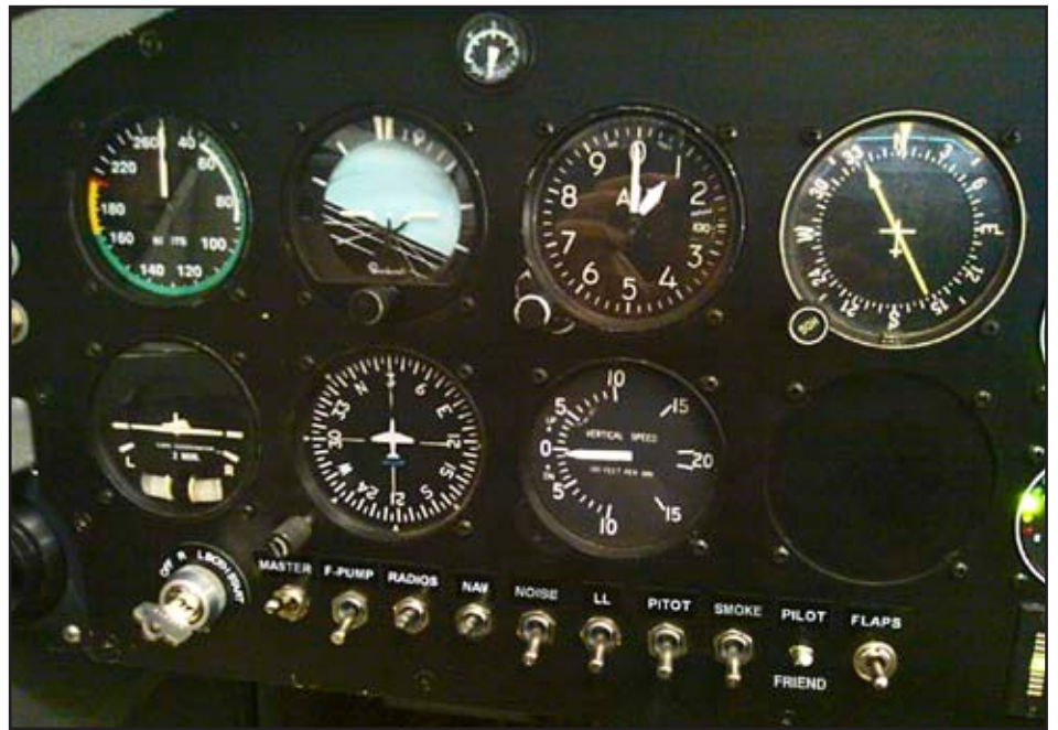
"Six-pack" flight instruments with ADF indicator and Switch/Breakers... Suction gauge above. It is not really a "Beechcraft" despite the Artificial Horizon logo. Yes that red line IS at 200kt (grin)
