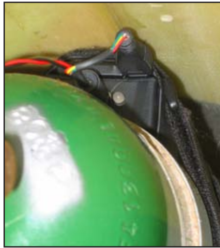
The APRS installed in a glider... strapped to the top of an oxy cylinder.
