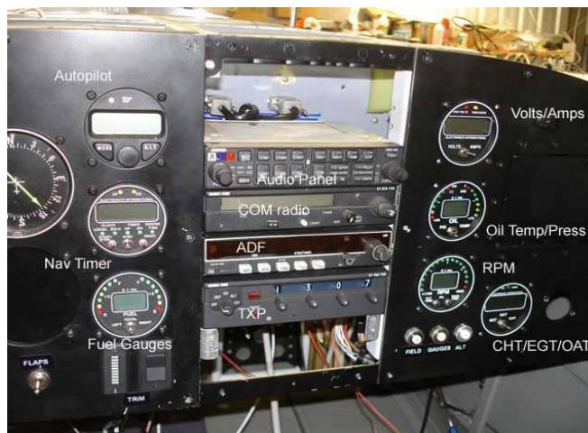
Radio stack – missing top panel above and throttle/mixture/carb heat cables below
